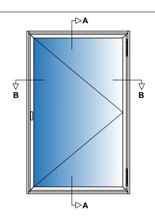
Aluminium 6063-T6 alloy to BS EN 755-9 standard, powder coated to BS 6496 to 60-80 micron finish.
