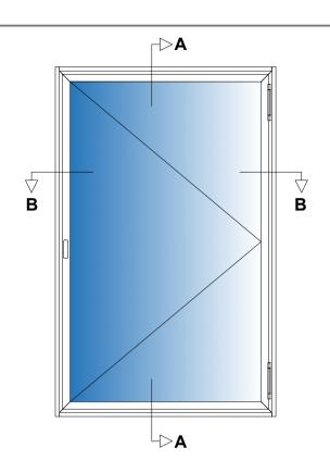
Aluminium 6063-76 alloy to BS EN 755-9 standard, powder coated to BS 6496 to 60-80 micron finish.
