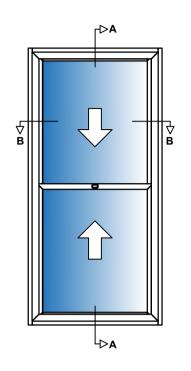
Aluminium 6063—76 alloy to BS EN 755—9 standard, powder coated to BS 6496 to 60 - 80 micron finish.
