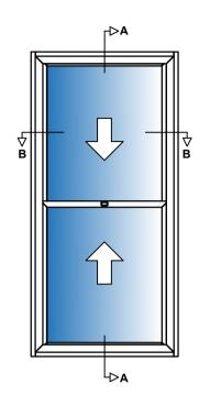
Aluminium 6063-T6 alloy to BS EN 755-9 standard, powder coated to BS 6496 to 60-80 micron finish.
