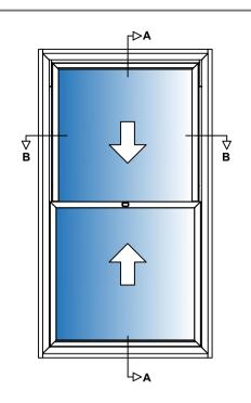
Aluminium 6063—T6 alloy to BS EN 755—9 standard, powder coated to BS 6496 to 60 - 80 micron finish.
