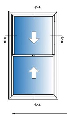
Aluminium 6063—76 alloy to BS EN 755—9 standard, powder coated to BS 6496 to 60 - 80 micron finish.
