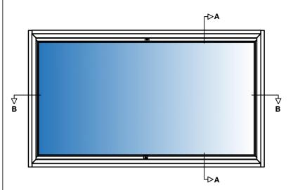
Aluminium 6063-T6 alloy to BS EN 755-9 standard, powder coated to BS 6496 to 60-80 micron finish.
