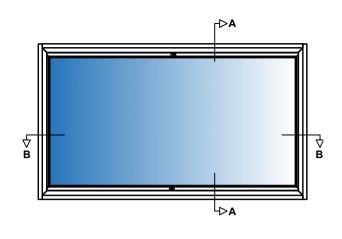
Aluminium 6063-T6 alloy to BS EN 755-9 standard, powder coated to BS 6496 to 60-80 micron finish.
