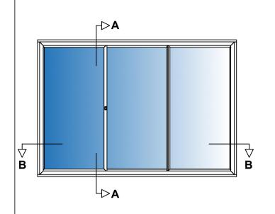
Aluminium 6063—T6 alloy to BS EN 755—9 standard, powder coated to BS 6496 to 60 - 80 micron finish.
