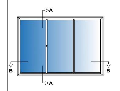
Aluminium 6063-T6 alloy to BS EN 755-9 standard, powder coated to BS 6496 to 60-80 micron finish.
