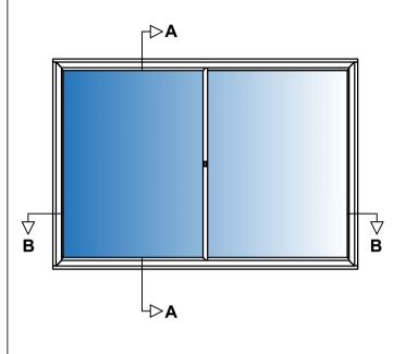
Aluminium 6063-T6 alloy to BS EN 755-9 standard, powder coated to BS 6496 to 60-80 micron finish.
